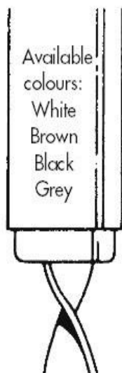
Available colours: White Brown Black Grey TYPE 'D' STANDARD 14mm DIAMETER TO SUIT 16mm x 16mm REBATE SASH WEIGHT UP TO 13.5kg
