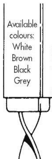
Available colours: White Brown Black Grey TYPE 'B' 12.4mm DIAMETER TO SUIT 14mm x 14mm REBATE SASH WEIGHT UP TO 13.5kg
